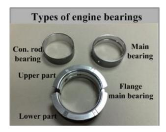
**Bearing** is a device supporting a mechanical element and providing its movement relatively to another element with minimum power loss.
